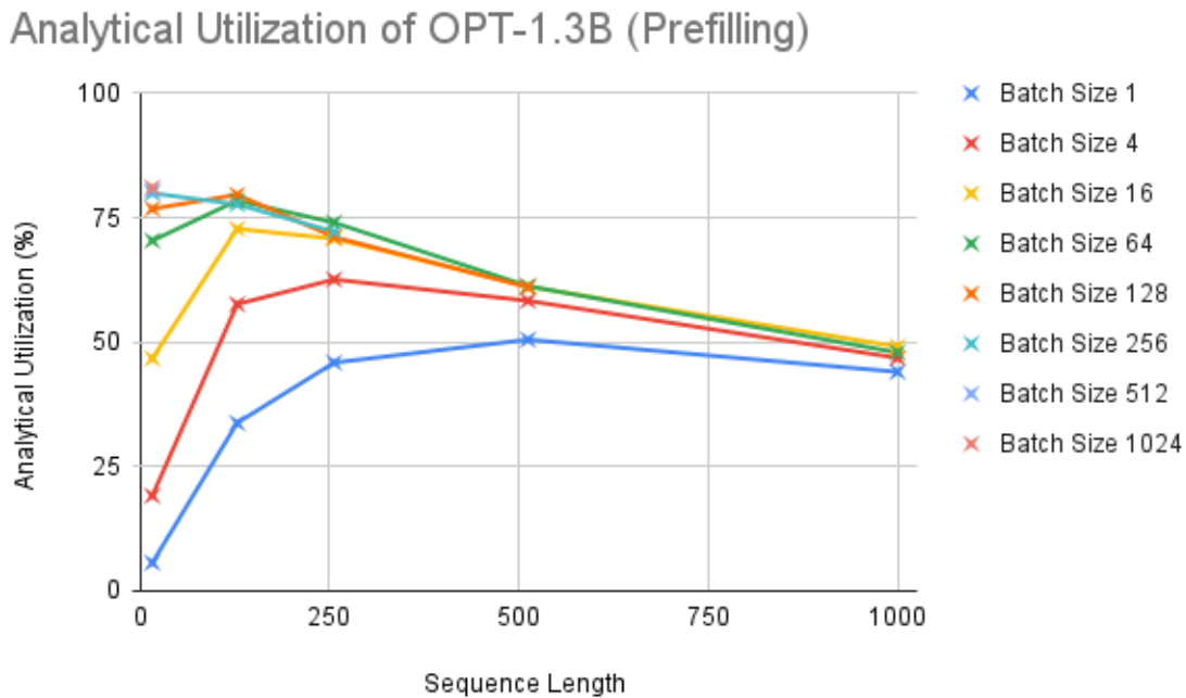
Figure 3-1: Analytical utilization (%) of OPT-1.3B during the prefilling stage for various batch sizes and input sequence lengths
